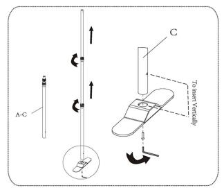
To insert pole #A-C into the socket of base vertically then tightening; Afterwards, screw off #A-C to the limited stop and screw up the plastic bolt.
