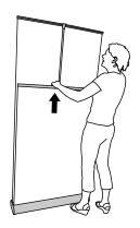
Step 2 Assemble the pole segments
