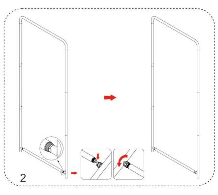
Using the big plastic screw parts to fasten the bottom cross bar
