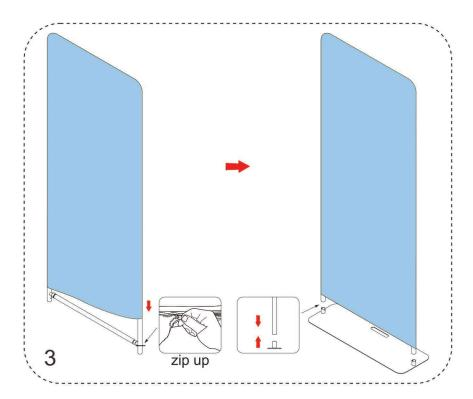
To wrap the fabric banner on the frame and zip up, afterwards install whole display stand to the base.
