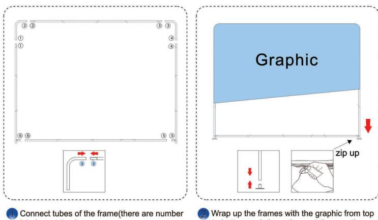
Connect tubes of the frame(there are number labels on tubes)
