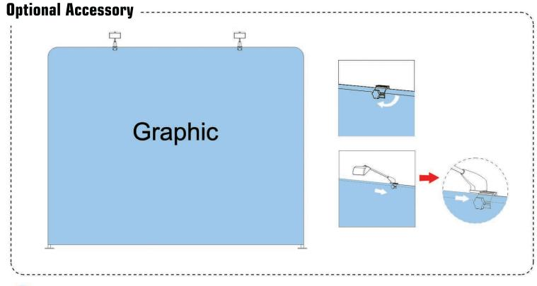
Put the light clip on the top of display and fix it with screw, then connect the light and the clip
